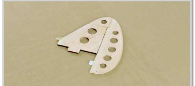
6.1 Place V2 and V3 on flat surface and apply glue to glue them together. Insert CA hinges to the vertical stabilizer hinge grooves, install rudder and check alignment of rudder. Do not apply glue to the CA hinges at this stage. Sand down rough edges if necessary.
