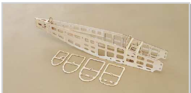
1.16 Press and fit right side fuselage to F4, F5, F5B, F16, F17, F20, F27 and landing gear housing, use tape to hold them in position.
