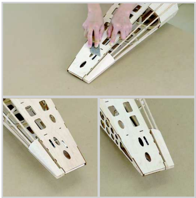
3.13 Cut and trim plastic sleeves to flush with fuselage.
