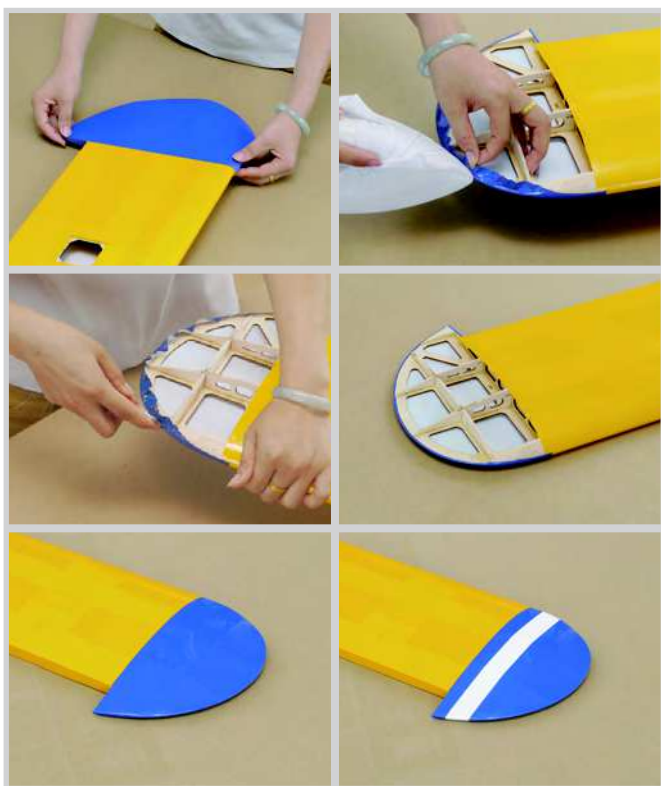
14.3 Cover wing tip, bottom first then the top. Apply higher heat to shrink covering around the round edges.
